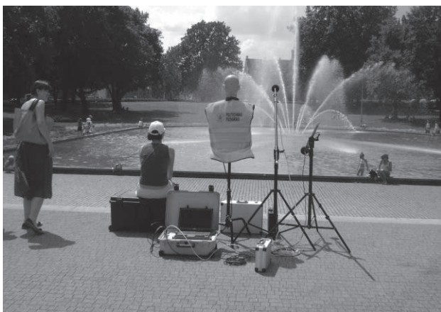
Figure 3: Example of a recording place for environmental signals necessary for the library of acoustic events and situations characteristic of a city life.
