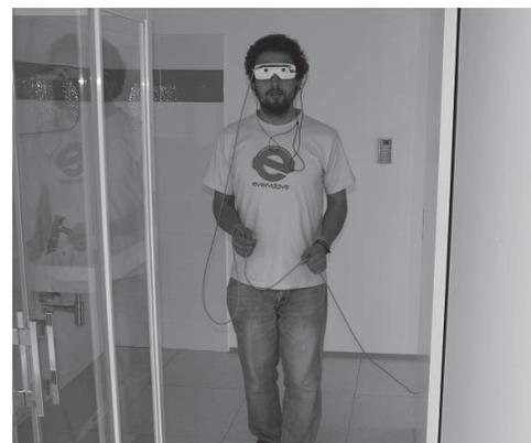
Figure 6. Blindfolded subject wearing navigation system nearly reaching the destination. Wired-base limitation of the system prototype is obvious.
