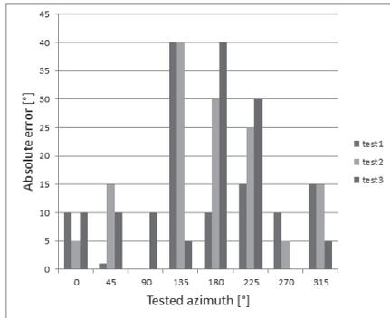
Figure 4. Bar chart showing the absolute localization error of the test subject during each of 3 test runs [9]
