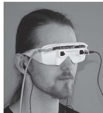
Figure 1. Subject wearing PERSEUS device with stereoscopic cameras and integrated headphones.
