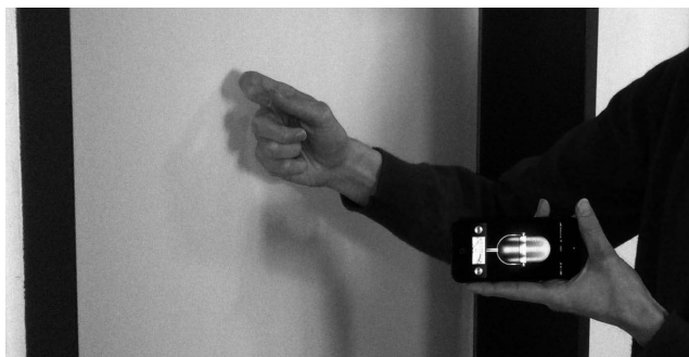
Figure 9: Someone in front of an office knocking at the door. The augmented knocking sound is recorded using the phone. A recording is available on our website http://www.techfak.uni-bielefeld.de/ags/ami/publications/TH2013-BSS
