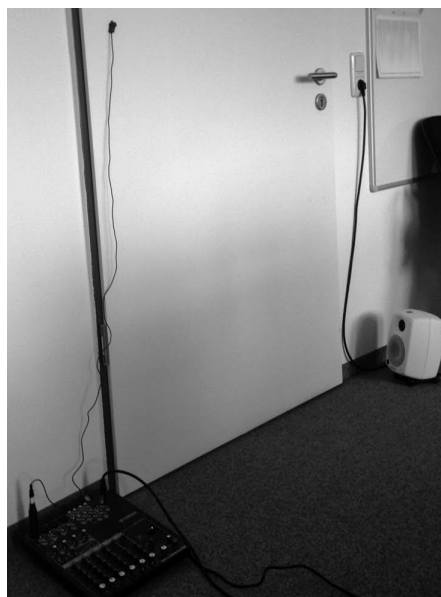
Figure 11: The Knock'Knock setup: A contact microphone is fixed at the door leaf. The signal is processed by SuperCollider3 on a computer (not shown in the image). The resulting sound is played back using the loudspeaker pointing towards the door.
