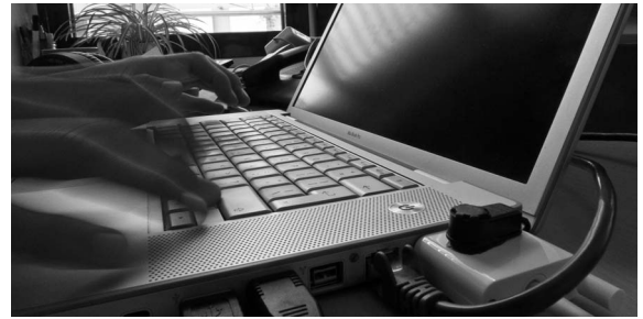
Figure 3: A setup used by participant in the augmented keyboard study. The transducer was attached to the external video adapter of her laptop. This made it easy for (dis-)assembly, since she only used the system only at her workplace, but carried her laptop with her
